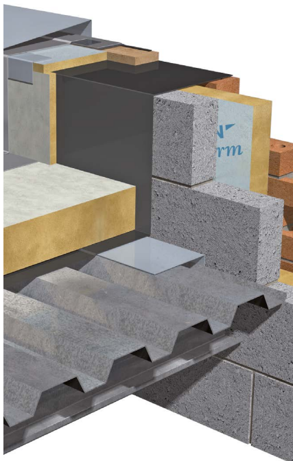
Flat roofs: QRFR-GFR in metal deck
