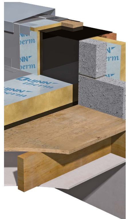
Flat roofs: QRFR-GFR in timber deck
